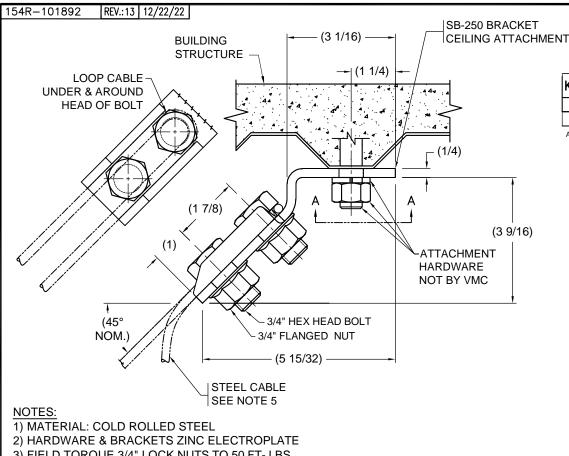
MAX. TENSION **KIT** KIT PART NUMBER "S" **COLOR CODE** ALLOWABLE **TYPE** 11/16" CLEAR ZINC COATED SB-250-01 4020 LBS. SLOT/HOLE 15/16" 11/16 CLEAR ZINC COATED 4400 LBS. HOLE SB-250-02
